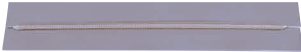
↑ Stainless steel (0.5 mm), Overlap fillet welding (same material) (Pulse current: 50A, Base current: 5A, Speed: 30cm/min.)
